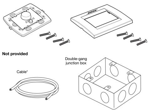
\*Shielded, data-grade cable (22-24 AWG or 0.34-0.25mm<sup>2</sup>) is recommended. Limit runs to 500 ft for shielded cable, 100 ft for unshielded.
